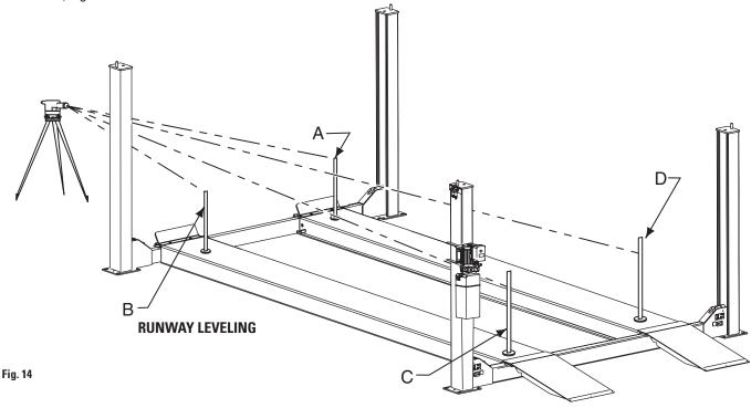
Note: Use a pencil, marking pen or attach a paper clip onto the target scale at the crosshair reference.
