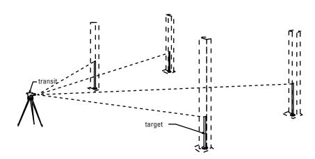
Dimension at highest position minus other position = shim thickness required
