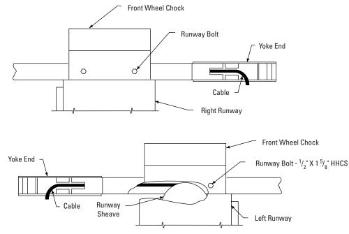
FEED CABLE ENDS THROUGH YOKE OPENINGS
