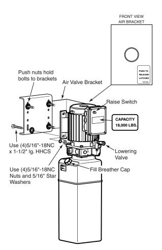
**MOUNTING AIR VALVE BRACKET** Fig. 17
