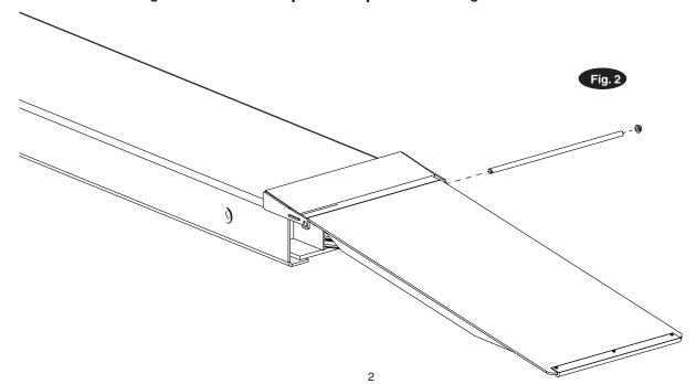
• Add 5/32" x 1" Lg. Cotter Pin to other side of pin assembly as shown, Fig. 3.
