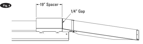
• Place Rear Steer Assembly adjacent to 19" Spacer. Parts should touch each other, Fig. 5.
