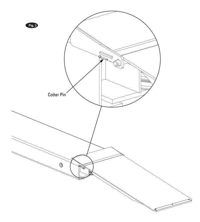
Note: Make sure lift is sitting on the floor or on the locks before removing the wheel stop
