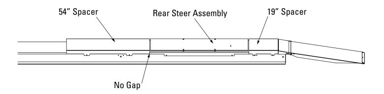
• Place 39" Spacer adjacent to 54" Spacer. Parts should have no gap. The Extended Length Alignment Kit receives one more 36" Spacer which also has a no gap, Fig. 7.
