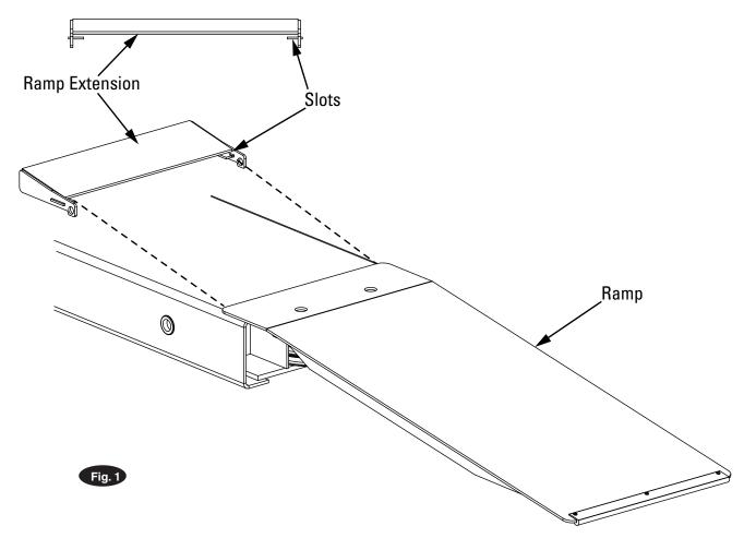
• Slide Ramp Extension down until the holes line up with holes in ramp and runway. Attach 5/8" Push Nut to Pin and slide it through both the Lift Ramp and Ramp Extension, Fig. 2.
